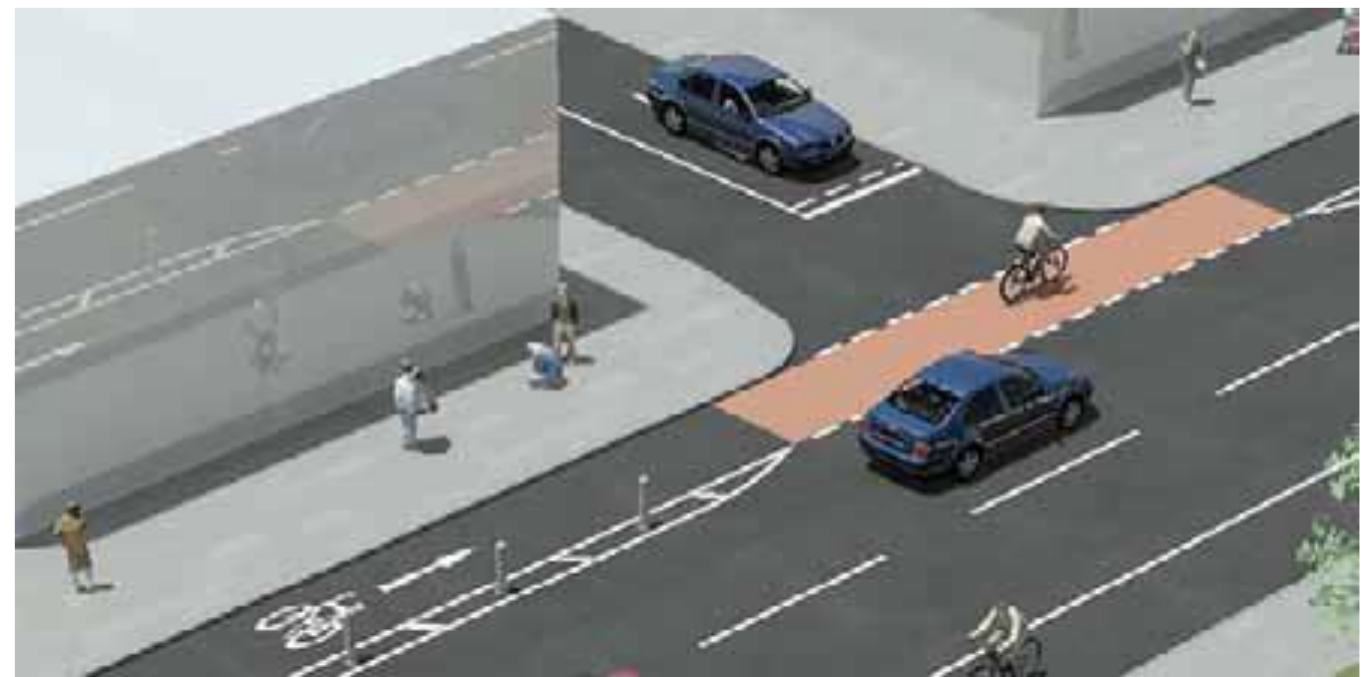
Figure 32: On-Road Cycle Lane Priority Junction Treatment
