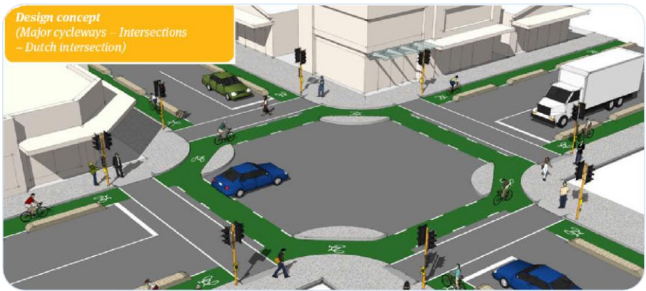
Figure 16: Key Infrastructure Elements of Protected Junction
