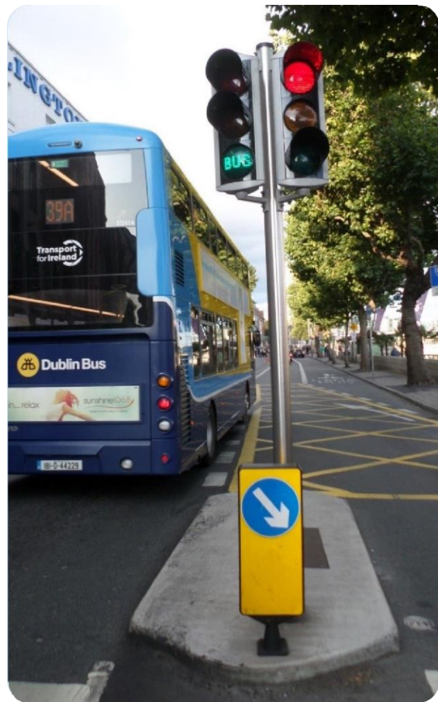
Figure 2: Signal Controlled Bus Priority
