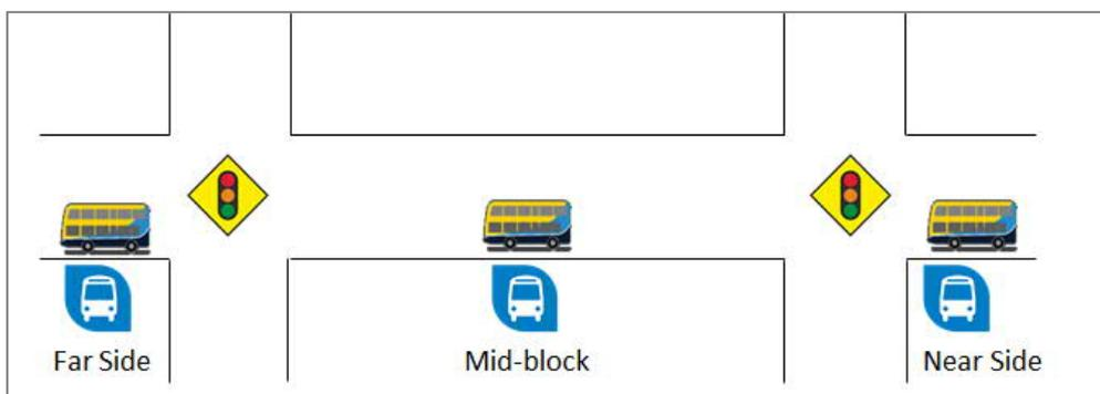
**Figure 1.4** Typical Location of Bus Stops.
