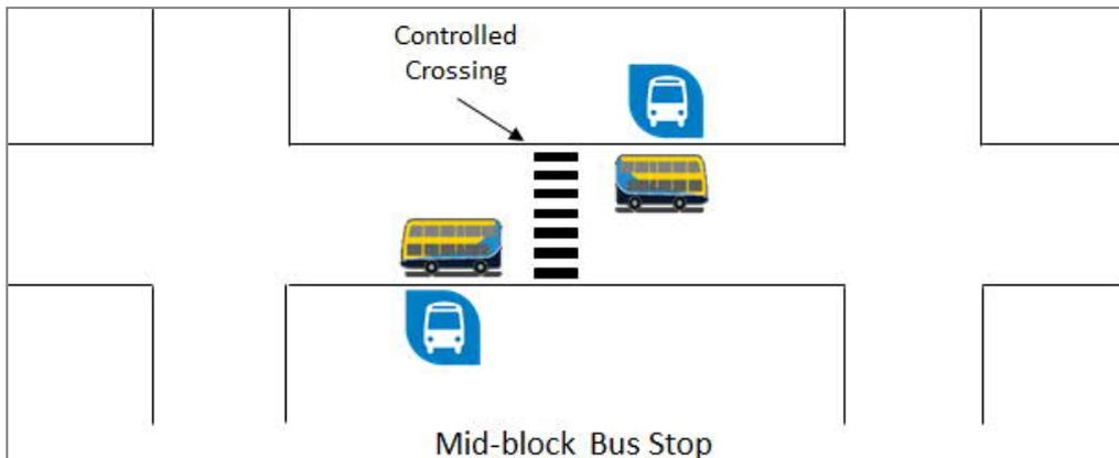
**Figure 5.10** Mid-block bus stop optimum layout.
