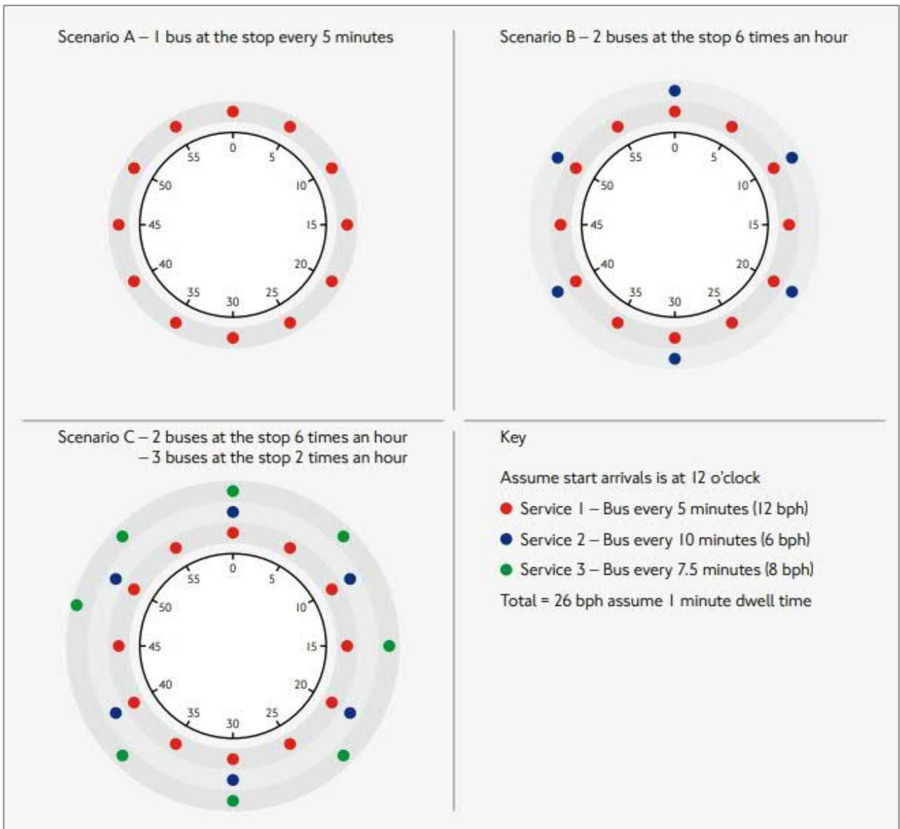
**Figure 7.1** Bus Arrival Pattern at a Bus Stop (Source: TFL Bus Stop Design Guidance)
